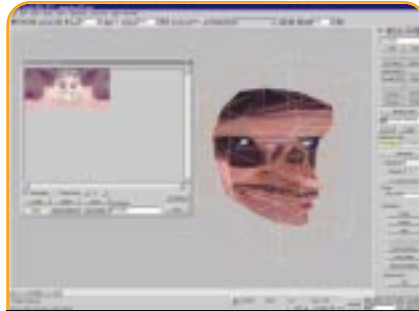
FIGURE 4. Switching from planar to cylindrical mapping in the middle of the operation isn't advisable.
